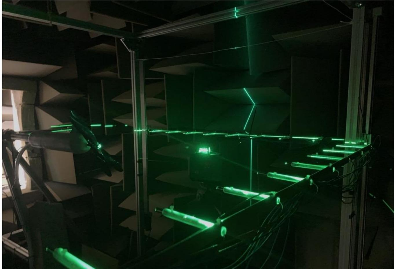
Microphone antenna alignment with shaft - ALCOVES
